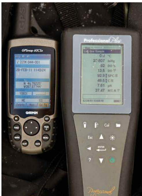
Old tech: A Garmin GPS unit verifying time and location of data collection alongside a handheld YSI meter, February, 2011. Photo by Chauncey Moran.
