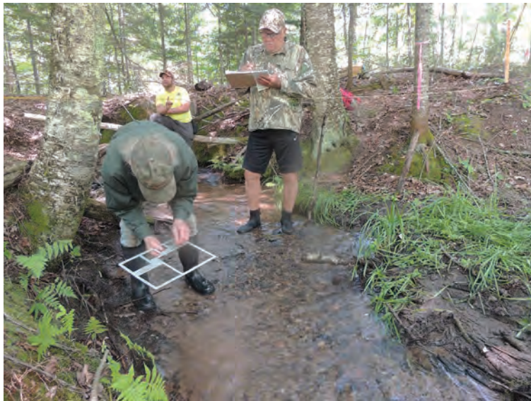
Jan Zender, Sam Prentice (background), and John Anderson conducting a pebble count. Photo by Ted Carland.
