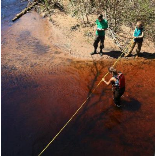
Figure 42 – Stream width and depth measurements taken at the County Road 510 bridge as part of the volunteer stream monitoring program.
